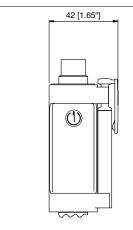
The Autozero function is activated through a magnetic contact (external magnet supplied with the sensor).
