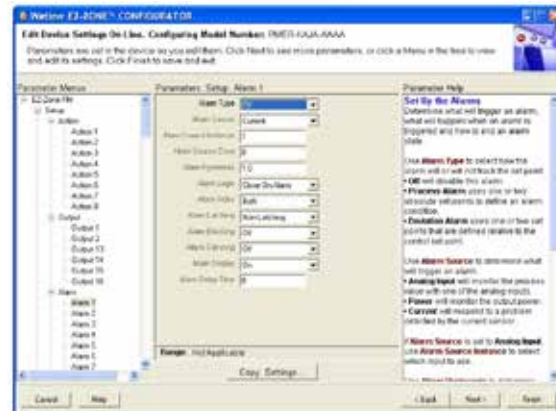
Menu explorer allows users to skip directly to desired parameter or browse each setting.
