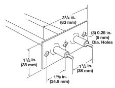
A 0.065 in. (1.7 mm) thick stainless steel bracket provides element mounting in non-pressurized applications. Attached to the heater sheath, these brackets are not suited for liquidtight mountings. The bracket is located ½ in. (13 mm) from the sheath's end, unless otherwise specified.
