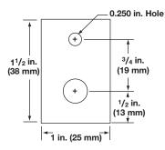
A 1½ in. (38 mm) x 1 in. (25 mm) wide x 16 gauge stainless steel bracket with one element hole and one mounting hole ½ in. (13 mm) from end.
