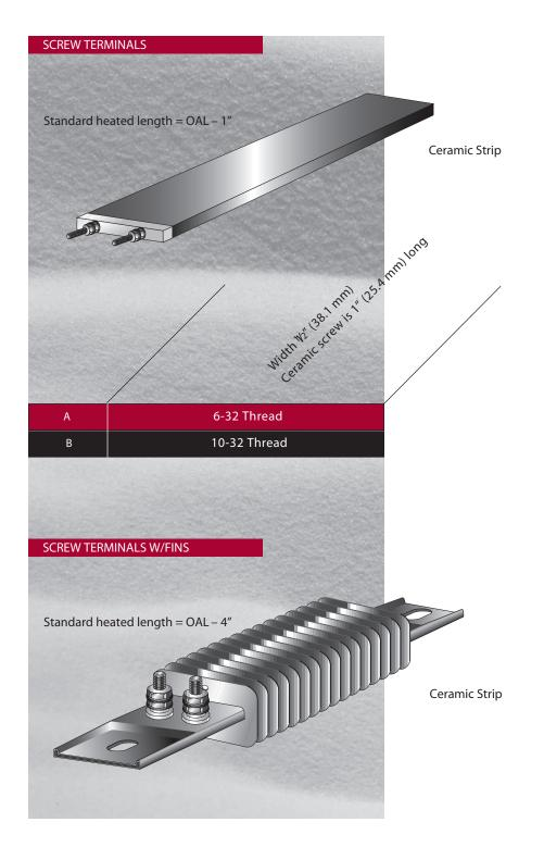
Simple-to-wire 6-32 stainless steel screw terminals arranged for maximum heated length, and for applications where lead access is only possible from one side and height clearance is a concern.
