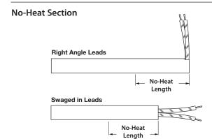
No-heat sections are recommended in applications where leads may be exposed to excessive heat, thus requiring a cooler lead end. Also use when heat is not required along the entire length of the metric FIREROD. No-heat extensions are available on all diameters with both pin style and swaged-in leads. To order, specify **no-heat** section and length of no-heat.
