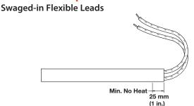
Swaged-in flexible leads, with silicone-fiberglass insulation, are recommended for applications in which the leads must be bent at the exit point from the heater. Unless longer length is specified, 250 mm (10 in.) leads are supplied.
