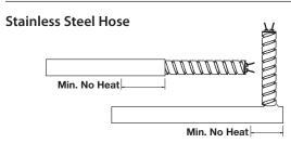
Stainless steel hose provides the best protection against abrasion from sharp edges or abrasive equipment. It also offers ease of handling and wiring in abrasive environments. When the leads exit at a right angle to the heater, the hose is silver soldered to the sheath. Unless otherwise specified, leads are 250 mm (10 in.) long and the hose is 200 mm (8 in.) long. To order, specify **stainless steel hose**, lead length and no-heat section.
