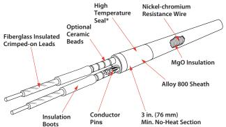
\* First 2 in. (51 mm) at lead end must be kept below 1000°F (538°C)
