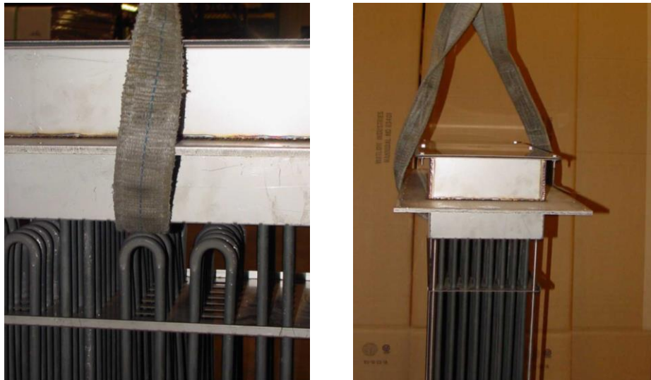
Figure 4 - For Vertical lifting place strap through the space between the element bundle and the insulation retainer. Do not slip the strap through the elements.
