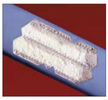
For 240VAC, 10kW wiring, only the outside coils of a FIREBAR would be wired, each coil providing 5kW. For 208VAC, 10kW wiring, all three coils would be wired; the outside coils providing 3.75kW each and the different resistance center coil 2.5kW.
