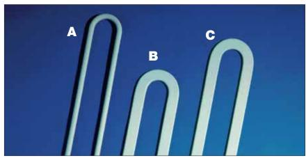
Although it is shorter, the FIREBAR element (heater B) provides the same wattage (800 watts) and watt density 23 W/in<sup>2</sup> (3.5 W/cm<sup>2</sup>) as the round tubular element (heater A). An equal length FIREBAR element (heater C) will provide more wattage (1360 watts) at the same watt density, or a lower watt density 13.5 W/in<sup>2</sup> (2.1 W/cm<sup>2</sup>) for 800 watts.
